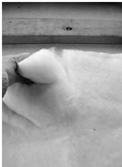
Left: Polyester batts tear easily for resizing – but in one direction only.
