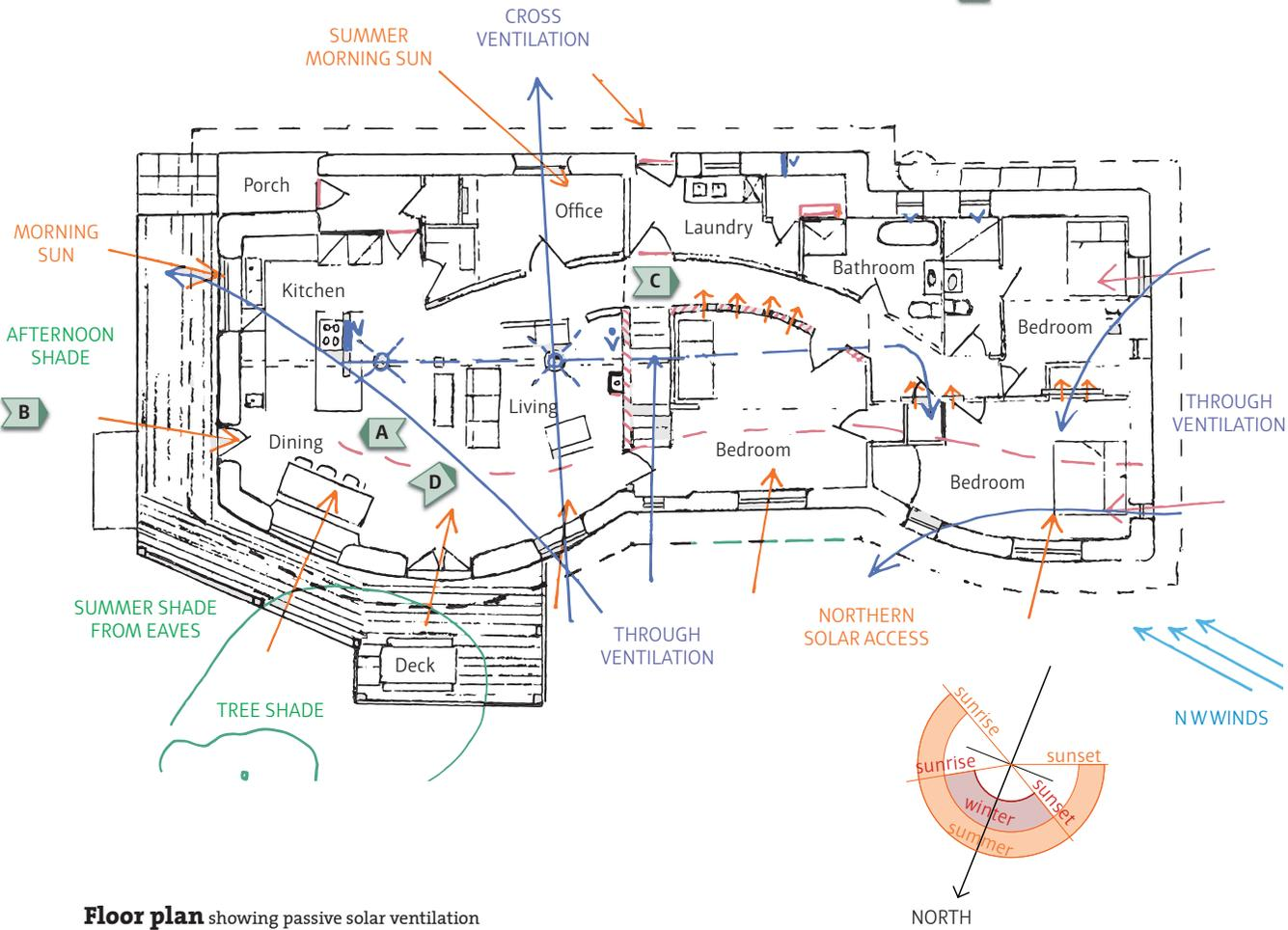
**Floor plan** showing passive solar ventilation
